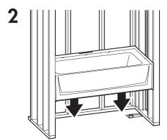
Check dimensions. **NOTE:** If you're adding additional accessories such as a grab bar–additional framing may be needed for support.
