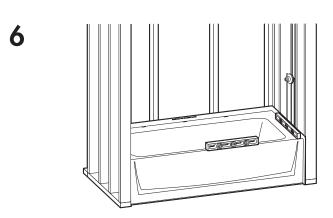
Level lengthwise and widthwise using 3 ft. (915mm) level by shimming if necessary. The unit must be set level.
