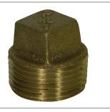
A.Y. M<sup>o</sup>Donald Mfg. Co. No-Lead Pipe Fittings & Nipples are constructed from heavy duty bronze and are rated for commerical, industrial and residential applications up to 125 WOG. Threads conform to ANSI B1.20.1 and fitting dimensions comply with ANSI B16.15.
