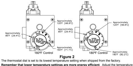
The thermostat dial is set to its lowest temperature setting when shipped from the factory. **Remember that lower temperature settings are more energy efficient.** Adjust the temperature by turning the thermostat dial. It is suggested that the starting point setting not be greater than the "\overline{2}" or "\overline{A}" mark on the thermostat dial (approximately 120°F [48.9°C]) as indicated above.
