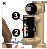
C. While holding the bypass valve open, use a wrench to turn the valve control stem (4) to adjust the flow rate slowly. The resulting flow rate is indicated by the metal ball (5) that slides up and down inside a transparent channel (6) marked by a graduated scale in gpm.
