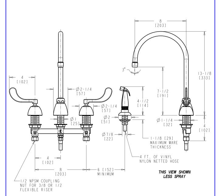
DIMENSIONS ARE IN INCHES AND [MILLIMETERS].
