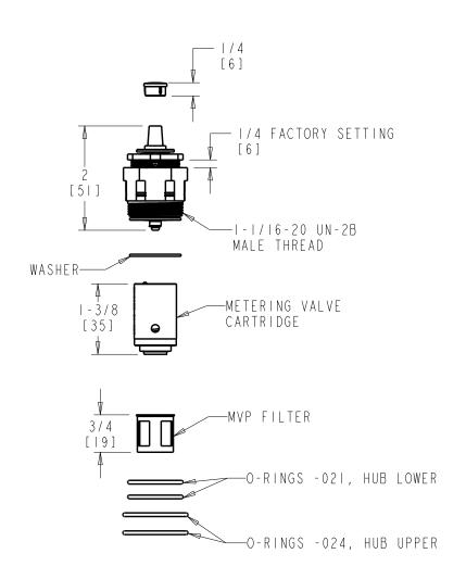
DIMENSIONS ARE IN INCHES AND [MILLIMETERS].
