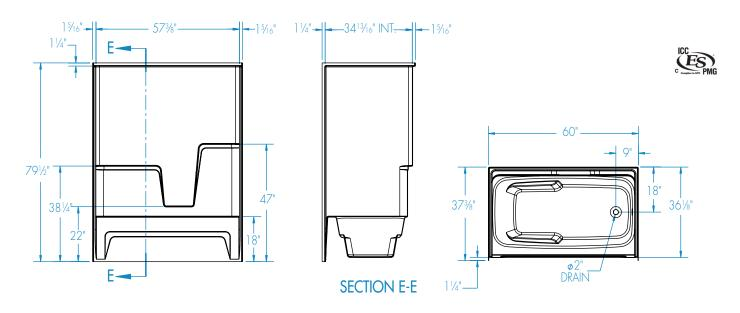
FEATURES Dimensional Tolerance ± 3/8". Dimensions needed for site preparation should be measured from the unit. Comfort Designs assumes no responsibility for preparatory work.
