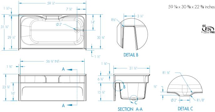
**FEATURES** Dimensional Tolerance ± %". Dimensions needed for site preparation should be measured from the unit. Comfort Designs assumes no responsibility for preparatory work.
