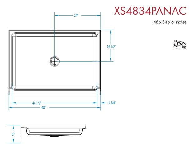
FEATURES Ibs Dimensional Tolerance ± 36". Dimensions needed for site preparation should be measured from the unit. Aquatic assumes no responsibility for preparatory work.
