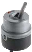
**OUR VALVE** Ceramic-on-ceramic valves traditionally use grease to maintain a frictionless surface for smooth handle motion. Over time, the calcium builds on the ceramic and the grease wears away, requiring extra effort to move the handle. Our patented diamond-on-ceramic design is not only greaseless, but actually polishes the ceramic with each use, keeping the operation like-new for life.
