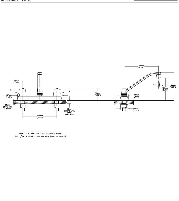
Delta reserves the right (1) to make changes to specifications and materials, and (2) to change or discontinue models, both without notice or obligation. Dimensions are for reference. Measurement may vary plus or minus 6mm(0.25"). Mounting locations are suggested only. Check with local codes for requirements in your area. This spec was produced May 26, 2017.
