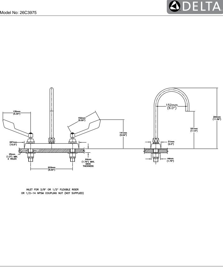
Delta reserves the right (1) to make changes to specifications and materials, and (2) to change or discontinue models, both without notice or obligation. Dimensions are for reference. Measurement may vary plus or minus 6mm(0.25"). Mounting locations are suggested only. Check with local codes for requirements in your area. This spec was produced May 25, 2017.
