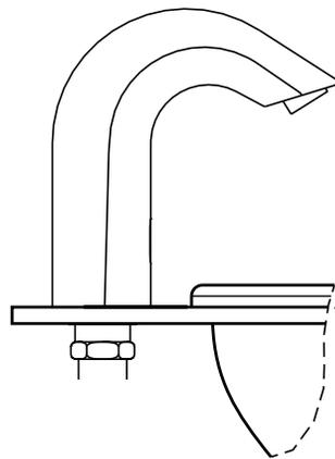
**For above deck mounted sinks, the sensor requires a clearance.**
