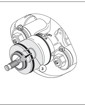
**C.** Make sure valve is in full cold position (to the right). Install adapter (5) to valve stem with stop lug positioned next to valve stop. Install extension (6). **Note: Extension (6) MUST be cut to length to accommodate desired handle position. (Install all components including handle and measure to determine desired cut length.)**
