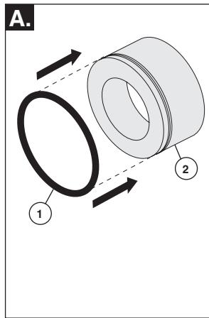
**A.** Assemble O-ring (1) to spacer (2).
