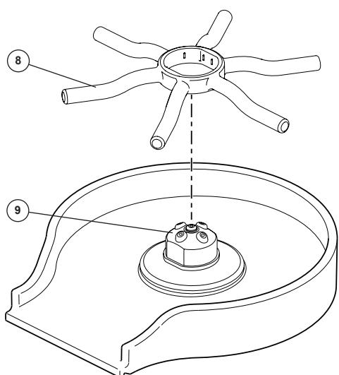
Align the locating features on the actuator arms (8) with those on the nozzle (9) and press actuator arms firmly into place on nozzle, oriented so the arms angle downward from the center. As needed, actuator arms can be removed for cleaning.
