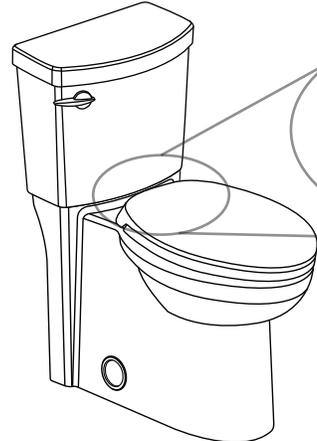
Put screws into seat hinge and tighten using a screwdriver.
