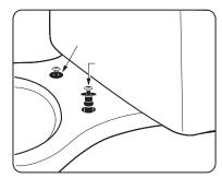
**NOTE:** FLANGE MUST REMAIN ABOVE THE SURFACE. DO NOT ALLOW GROMMET TO FALL THROUGH!
