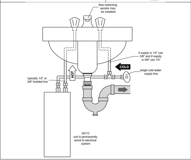
**4.** Open the hot water faucet and run water for minimum 60 seconds and until the flow is continuous and free of air pockets. Close the faucet and install the aerator (if supplied).
