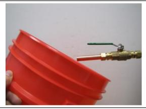
**2.** Make sure the inlet filter screen is present in the inlet fitting and the inlet and outlet pipes are correctly aligned with the heater connections to minimize stress on the heater.
