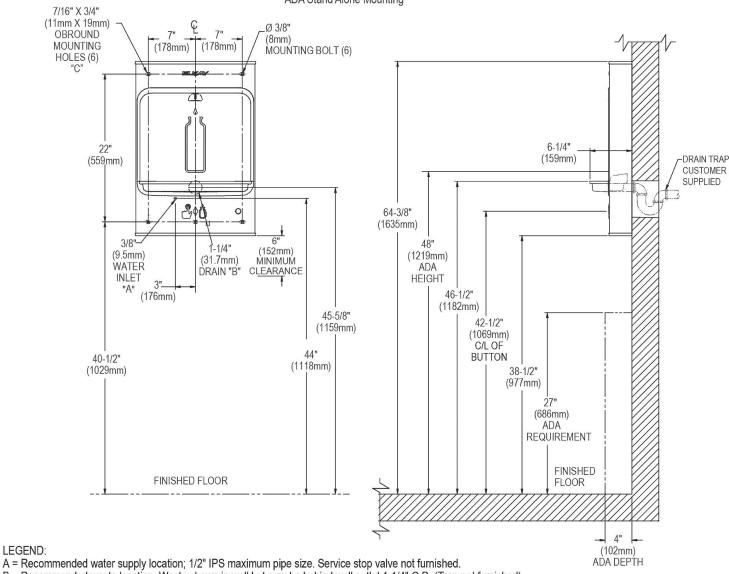
B = Recommended waste location. Waste shown in wall but may be behind wall outlet 1-1/4" O.D. (Trap not furnished).
