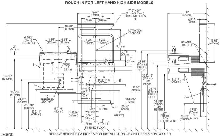
A = Recommended Water Supply location. Shut-off Valve (not furnished) to accept 3/8" O.D. unplated copper tube. Up to 3" (76mm) maximum out from wall. B = Recommended Waste Outlet location. To accommodate 1-1/2" nominal drain. Drain stub 2" (51mm) out from wall.
