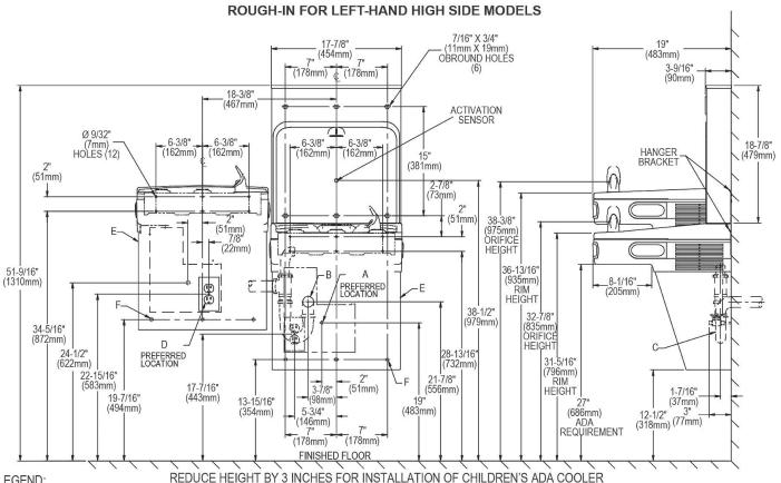
LEGEND: A = Recommended Water Supply location. Shut-off Valve (not furnished) to accept 3/8" O.D. unplated copper tube. Up to 3" (76mm) maximum out from wall. B = Recommended Waste Outlet location. To accommodate 1-1/2" nominal drain. Drain stub 2" (51mm) out from wall.
