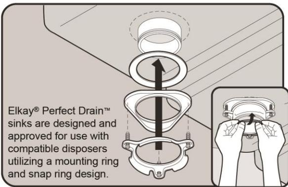
Elkay<sup>®</sup> Perfect Drain<sup>™</sup> sinks are designed and approved for use with compatible disposers utilizing a mounting ring and snap ring design.
