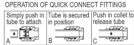
Pushing tube in before pulling it out helps to release tube
