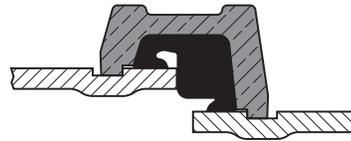
**Reducing Coupling Gasket:** This gasket is provided with ribs used to position the larger pipe so that the sealing lip is located on the sealing surface of the pipe. This gasket is used only with the GRINNELL Figure 716 Reducing Coupling.
