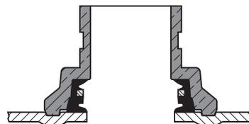
**Outlet Coupling Gasket:** This gasket is specifically designed for use with the GRINNELL Figure 702 Outlet Coupling.
