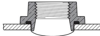
**Mechanical Tee Gasket:** This gasket provides a compression type seal, which is designed to conform to the exterior curve (OD) of the pipe. Use this type of gasket ONLY with Figure 730 Mechanical Tees and Crosses.
