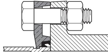
**Flange Adapter Gasket:** This gasket is specifically designed for use with GRINNELL Flange Adapters. The gasket has an optimal amount of rubber to provide a dependable seal between both the pipe and mating surface.
