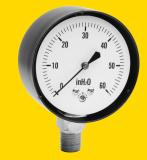
Trerice Low Pressure Gauges are essential for accurately measuring low pressures such as natural gas. This gauge employs a diaphragm capsule element to accurately measure pressures of 10 psi or below. The case is drawn steel with brass wetted parts.
