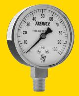
The Trerice 800B Utility Gauge is designed for general pressure indication requirements. This gauge provides excellent accuracy (1.6% full scale) and reliability at an economical cost. The case is drawn steel and wetted parts are brass.
