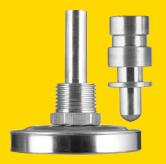
The Trerice "Econo-Met" thermometer is both an accurate and cost effective way to measure hot water in hydronic systems. The 2" stem makes this the ideal instrument for applications where there are space restrictions. An included 1/2 NPT brass thermowell or 3/4" brass sweatwell provide alternate ways for installation.
