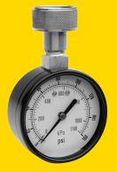
Trerice Gas and Water Test Gauges are integral tools for passing building inspections. Once the system has been pressurized, any leaks are visible as a pressure drop on the dial of the Gas Test Gauge. The Water Test Gauge has a 3/4 NPT hose bib connection mounted at 12 o'clock for easy viewing and accurately measures in-line water pressure. A maximum register pointer is available on either gauge having a dial range of 60 psi or greater.
