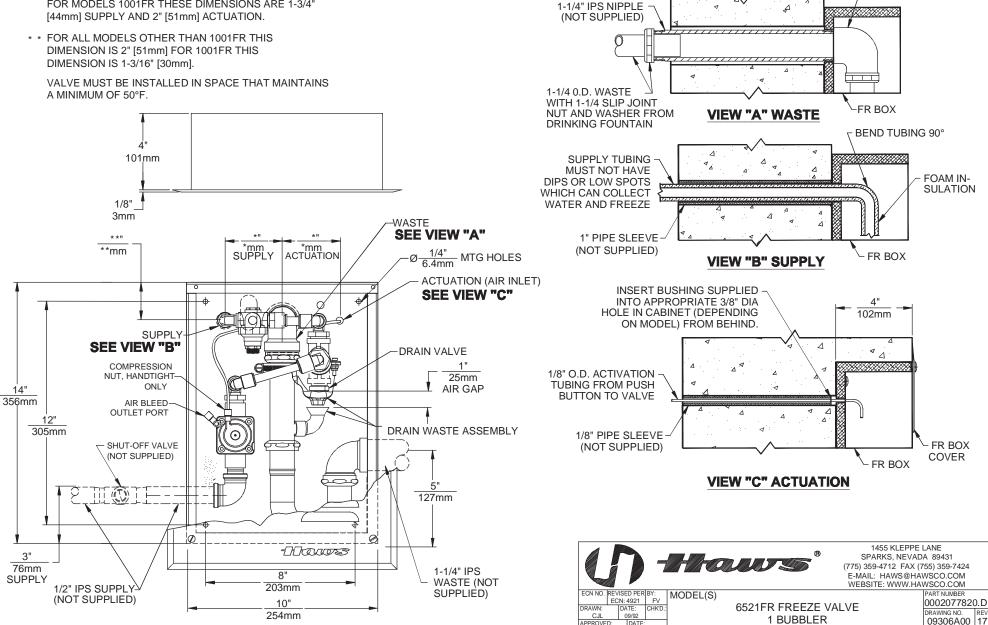
1-1/4 IPS X 1-1/4 O.D. ELBOW TO DRAIN WASTE
