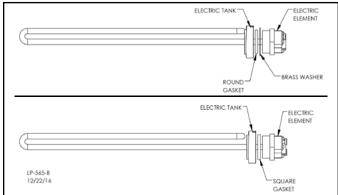
Figure 7 - Heating Element Detail
