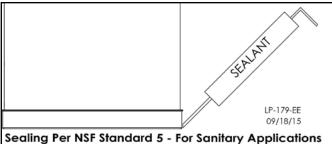
Apply a 3/8" bead of RTV Silicone completely around the tank to seal the base to the floor and prevent seepage underneath.
