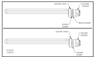
Figure 8 - Heating Element Detail
