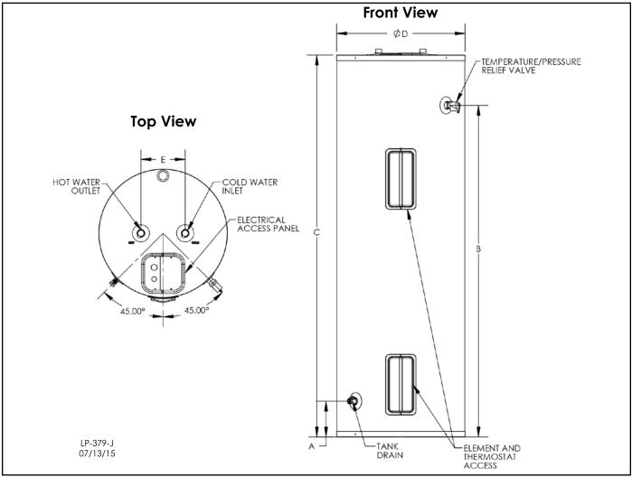
Figure 2 - Dimensional Drawing - Staged Operation
