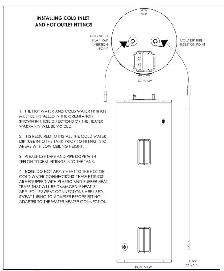
Figure 4 - Installing Cold Inlet and Hot Outlet Fittings
