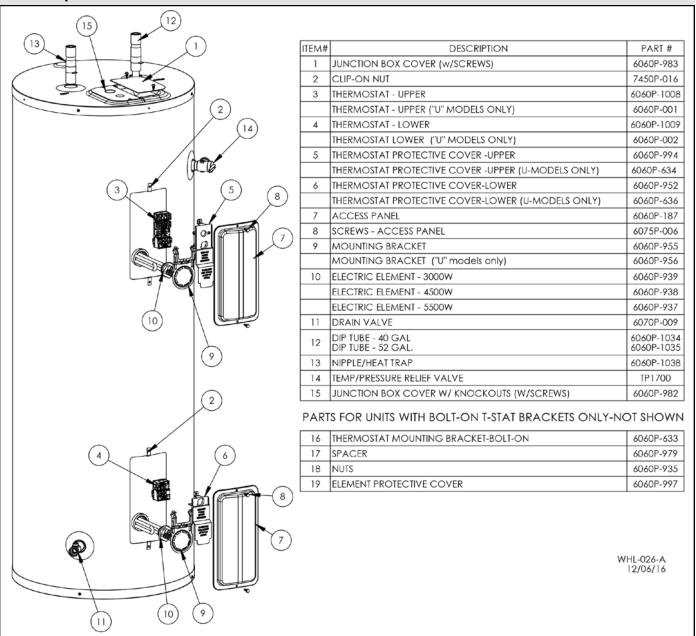
Figure 9 - Replacement Parts - Staged Operation
