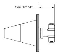
The TESTRITE® TRW2 through TRW6 (TEST WEDGES) are used in conjunction with TESTRITE TEE'S, which allow temporary blocking of the DWV stack for testing. Available in 2", 3", 4" & 6".
