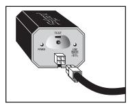
Plug wire harness into connector on face of control.
