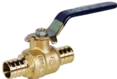
Maintenance-free dual EPDM® O-ring stem seal, zinc plated steel handle with vinyl cover CWP 400 PSI, ASTM F1806. Third party certified no lead ANSI/NSF 61-G & ANSI/NSF 14, IAPMO. Configuration and Sizes: PEX x DZR PEX, 1/2" - 1-1/4".
