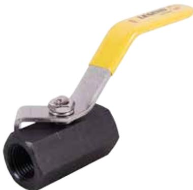
Heavy-duty one-piece carbon steel barstock body. Bottom-loaded blowout-proof stem, 304 stainless steel handle & nut, stem and ball. Ideal for commercial or industrial applications where port size is not critical. Available in sizes and configurations 1/4" - 2", FNPT x FNPT.
