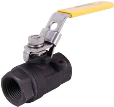
Heavy-duty two-piece carbon steel investment cast body and end adaptor. Bottom-loaded blowout-proof stem, 316 stainless steel ball and stem, 304 stainless steel latch-lock handle and trim. Fiber reinforced graphite impregnated seats maintain their shape in high pressure service. Integral, tapped mounting pad for actuation or panel attachment. Ideal for commercial or industrial applications. Available in sizes & configurations: 1/4" - 2", FNPT x FNPT.
