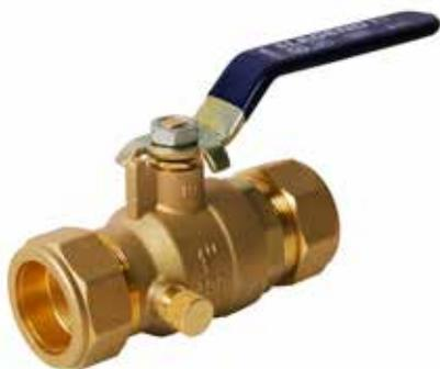
Full port ball valve with drain and compression ends for convenient installation onto copper tubing. Constructed of no lead binary brass. Configuration and Sizes: Compression x Compression 1/2", 3/4", & 1". Third party certified no lead ANSI/NSF 61-G, IAPMO.
