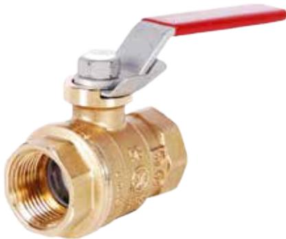
Maintenance-free, dual Viton® O-ring stem design, lighter weight and durable forged traditional brass body, blow-out proof stem, PTFE seats for improved wear. Dacromet® coated steel handle and nut for greater corrosion resistance with Dacromet® coated steel lock shield that includes eyelet for padlock. Available in sizes and configurations 1/2" - 2", FNPT x FNPT.
