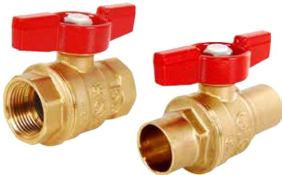
Maintenance-free, dual Viton® O-ring stem design, lighter weight and durable forged traditional brass body, blow-out proof stem, PTFE seats for improved wear. Coated cast aluminum tee handle that is light weight and compact in size. Available in sizes and configurations 1/2" x 1", FNPT x FNPT and 1/2" - 1", Sweat x Sweat.
