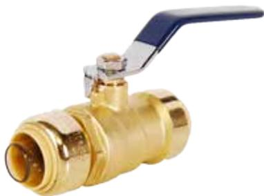
Push fit connect ends can be installed onto copper, PEX or CPVC. Insert stiffeners are included for use with PEX tubing. Configuration and Sizes: PTC x PTC 1/2", 3/4", & 1". CWP 200 PSI. Third party certified no lead ANSI/NSF 61-G & DZR ANSI/NSF 14, IAPMO. ASSE 1061.
