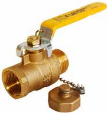
Traditional forged brass full port ball valve, 3/4" FNPT x 3/4" GHT. Garden hose includes GHT cap with gasket and tethered to valve end. \*Capped GHT connection is rated 125 PSI.
