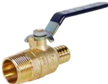
Maintenance-free dual EPDM® O-ring stem seal, zinc plated steel handle with vinyl sleeve. Third Party certified no lead ANSI/NSF 61-G & DZR ANSI/NSF 14, IAPMO. CWP 400 PSI. ASTM F1806. Configuration and Sizes: MNPT x PEX, 1/2" - 1".
