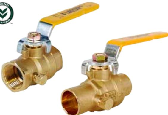
Forged no lead brass full port ball valve, bottom load blow-out proof stem with PTFE packing gland and nut. Drain for maintenance and freeze protection. Constructed of no lead binary brass alloy. Does not require any additional steps to solder, as compared to traditional brass valves. Suitable for potable water applications. Available in sizes and configurations 1/2" - 1", FNPT x FNPT and 1/2" - 1", Sweat x Sweat.
