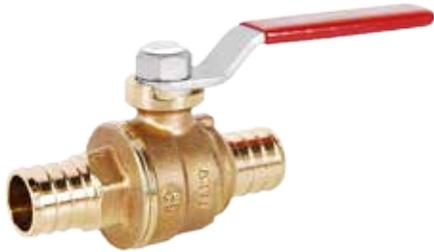
Maintenance-free dual Viton® O-ring stem seal, Dacromet® coated steel handle, CWP 400 PSI, ASTM F1806 PEX Ends. Third party certified no lead ANSI/NSF 61-G, NSF. Configuration and Sizes: PEX x PEX, 3/8" - 1".
