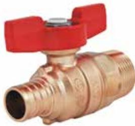
Maintenance-free dual Viton® O-ring stem seal, coated cast aluminum handle, CWP 400 PSI, ASTM F1806. With coated cast aluminum tee handle. Third party certified no lead ANSI/NSF 61-G, NSF. Configuration and Sizes: MNPT x PEX, 1/2" & 3/4".
