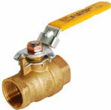
Traditional brass full port ball valve, bottom-loaded blow-out proof stem with PTFE packing gland and nut, 304 stainless steel ball and stem which are stronger and ideal for more heavy use, more frequent operation. Chrome plated steel handle with locking mechanism, eyelet for padlock. Available in sizes and configurations 1/2" - 2", FNPT x FNPT.
