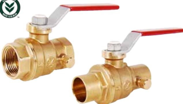
Maintenance-free, dual Viton® O-ring stem design, light weight and durable forged no lead brass body, blow-out proof stem, PTFE seats for improved wear. Ball with drain for maintenance or to prevent freeze. Dacromet® coated steel handle and nut for greater corrosion resistance. Constructed of no lead binary brass alloy. Suitable for potable water applications. Available in sizes and configurations 1/2" - 1", FNPT x FNPT and 1/2" - 1", Sweat x Sweat.
