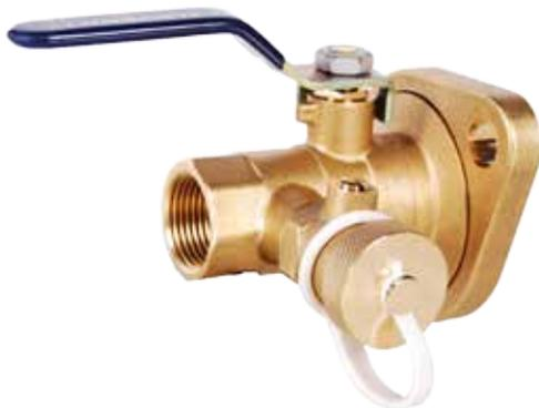
Traditional forged brass full port ball valve with flanged end and integrated drain valve for isolating circulator pumps. Standard flange connection rotates for positioning valve. Mounting holes are elongated to fit high velocity pumps. 1/4- turn tool activated drain valve with 3/4" GHT end and tethered brass cap. Configuration and Size: FNPT x Flange, Sweat x Flange, and 3/4", 1" and 1-1/4".
