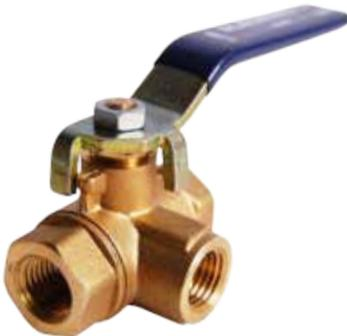
Traditional forged brass full port ball valve diverts media to the side-leg connection from either run connection. Directional arrow on handle indicates flowpath. Configurations and Sizes: FNPT x FNPT x FNPT, 1/4" - 2".
