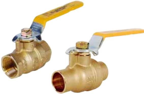
Forged traditional brass full port ball valve, bottom load blow-out proof stem with PTFE packing gland and nut. Available in sizes and configurations 1/4" - 3", FNPT x FNPT and 3/8" - 3", Sweat x Sweat.
