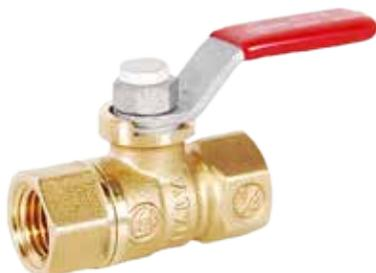
Traditional forged brass, compact body, mini-ball valve with Dacromet® coated steel handle, vinyl cover. Configurations and Sizes: FNPT x FNPT, 1/8" - 1/4".
