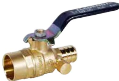
Maintenance-free dual EPDM® O-ring stem seal, zinc plated steel handle with vinyl sleeve CWP 400 PSI, with drain. Third Party certified no lead ANSI/NSF 61-G & DZR ANSI/NSF 14, IAPMO. ASTM F1806. Configuration and Sizes: Sweat x PEX, 1/2" - 1".
