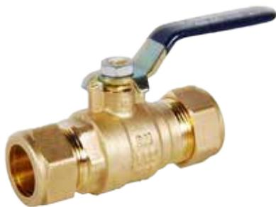
Full port ball valve with compression ends for convenient installation onto copper tubing. Constructed of no lead binary brass. Configuration and Sizes: Compression x Compression, 1/2", 3/4", & 1". Third party certified no lead ANSI/NSF 61-G, IAPMO.
