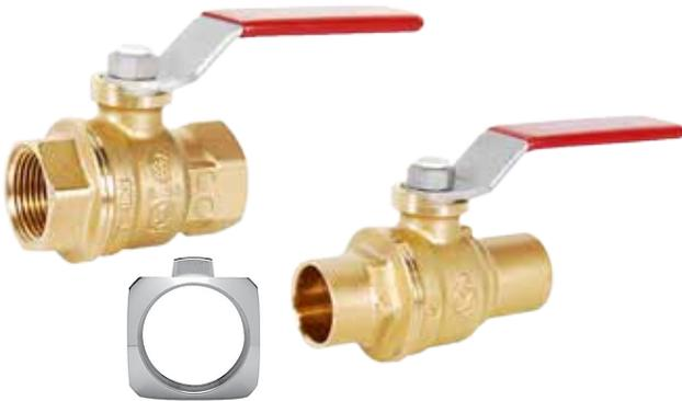
Forged body and end adapters are oversized. Large body with large wrench flats. Available in sizes and configurations 1/2" - 4", FNPT x FNPT and 1/2" - 3" Sweat x Sweat.
