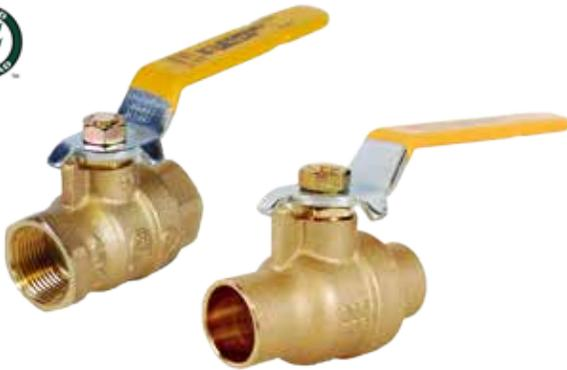
Forged no lead brass full port ball valve, bottom load blow-out proof stem with PTFE packing gland and nut. Constructed of no lead binary brass alloy. Suitable for potable water applications. Does not require any additional steps to solder, as compared to traditional brass valves. Available in sizes and configurations 1/4" - 3", FNPT x FNPT and 3/8" - 3", Sweat x Sweat.
