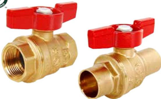
Maintenance-free, dual Viton® O-ring stem design, lighter weight and durable forged no lead brass body, blow-out proof stem, PTFE seats for improved wear. Coated cast aluminum tee handle that is light weight and compact in size. Available in sizes and configurations 1/2" x 1", FNPT x FNPT and 1/2" - 1", Sweat x Sweat.
