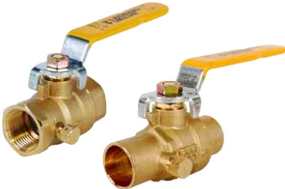
Forged traditional brass full port ball valve, bottom load blow-out proof stem with PTFE packing gland and nut. Drain for maintenance and freeze protection. Available in sizes and configurations 1/2" - 1", FNPT x FNPT and 1/2" - 1", Sweat x Sweat.
