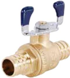
Maintenance-free dual EPDM® O-ring stem seal, zinc plated steel tee handle, CWP 400 PSI, Third Party certified no lead ASNI/NSF 61-G & DZR ANSI/NSF 14, IAPMO. ASTM F1806. Configuration and Sizes: PEX x PEX, 1/2" - 3/4".
