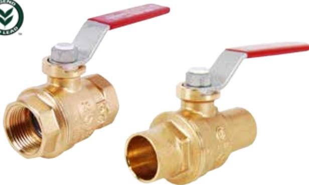
Maintenance-free, dual Viton® O-ring stem design, lighter weight and durable forged no lead brass body, blow-out proof stem, PTFE seats for improved wear. Does not require any additional steps to solder, as compared to traditional brass valves. Suitable for potable water applications. 1/8" - 4", FNPT x FNPT and 1/2" - 4", Sweat x Sweat.
