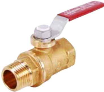
No lead forged brass mini-ball valve, with Dacromet® coated steel handle has vinyl cover. Configurations and Sizes: MNPT x FNPT, 1/8" - 1".
