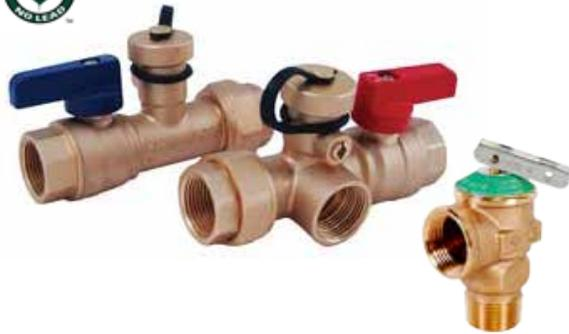
Hot and cold water heater isolation valves and pressure relief valve. No lead brass full port ball valves, include 150 PSI pressure relief valve. Tethered cap on tool activated drain valves integral in body of each valve, hot and cold. Configuration and Size: FNPT (Captive Union) X FNPT, Sweat (Captive Union) X Sweat, 3/4" x 3/4", & 1" x 1".
