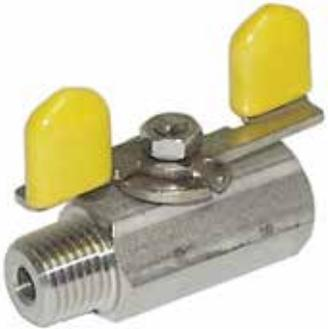
One-piece cast 316 stainless steel body, 304 stainless steel T-handle. Available in 1/4" MNPT x FNPT.
