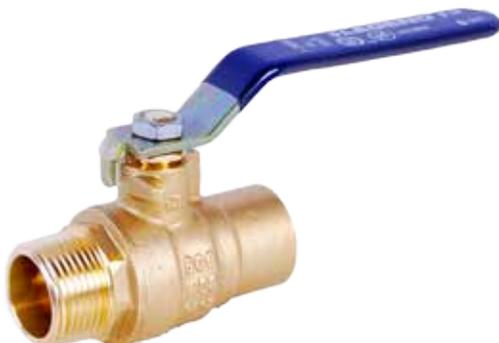
No lead forged brass full port ball valve for transitioning from a tank or boiler directly to copper tube. Configuration and Size: MNPT x Sweat, 3/4" x 3/4".
