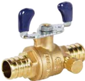
Maintenance-free dual EPDM® O-ring stem seal, zinc plated steel tee handle, CWP 400 PSI, with drain. Third Party certified no lead ANSI/NSF 61-G & DZR ANSI/NSF 14, IAPMO. ASTM F1806. Configuration and Sizes: PEX x PEX, 1/2" - 1".
