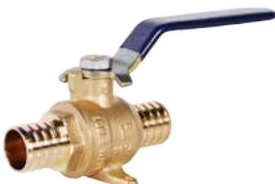
Maintenance-free dual EPDM® O-ring stem seal, zinc plated steel handle with vinyl sleeve and drop ears. CWP 400 PSI. Third Party certified no lead ANSI/NSF 61-G & DZR ANSI/NSF 14, IAPMO. ASTM F1806. Configuration and Sizes: PEX x PEX, 1/2" - 1".
