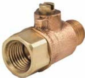
No lead cast brass test cock ball valve, with screwdriver slot stem for actuation. Configurations and Sizes: FNPT x MNPT, (1/4" x 1/8") & (1/4" x 1/4").
