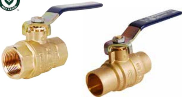
The T/S-2000NL no lead brass full port ball valve has a larger pattern body suitable for most any application. Constructed of no lead & DZR binary brass alloy. Available in sizes and configurations 1/4" - 4", FNPT x FNPT and 1/2" - 4", Sweat x Sweat.
