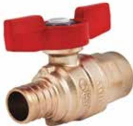
Maintenance-free dual Viton® O-ring stem seal, coated cast aluminum handle, CWP 400 PSI, ASTM F1806 PEX Ends. With coated cast aluminum tee handle. Third party certified no lead ANSI/NSF 61-G, NSF. Configuration and Sizes: Sweat x PEX, 1/2" & 3/4".
