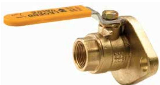
Traditional forged brass full port ball valve with flanged end for isolating circulator pumps. Configuration and Size: FNPT x Flange, Sweat x Flange, and 3/4", 1" and 1-1/4".
