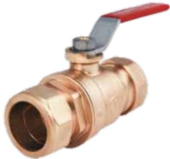
Maintenance-free dual o-ring full port ball valve with compression ends for convenient installation onto copper tubing. Constructed of no lead binary brass. Configuration and Sizes: Compression x Compression, 1/2", 3/4", & 1". Third party certified no lead ANSI/NSF 61-G, NSF.
