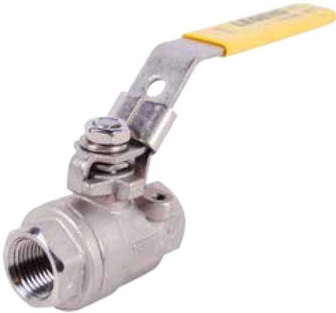
Heavy-duty two-piece investment cast body design, 316 stainless steel body & end adaptor. Bottom-loaded blowout-proof stem. Equipped with a latch-lock handle, 304 stainless steel trim, 316 stainless steel stem and ball. Ideal for commercial and industrial applications. Fiber reinforced, graphite impregnated seats maintain their shape in high pressure service. Integral, tapped mounting pad for actuation or panel attachment. Available in sizes & configurations: 1/4" - 2", FNPT x FNPT.
