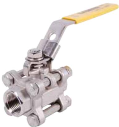
Heavy-duty three-piece investment cast body design, 316 stainless steel body & adaptors. Bottom-loaded blowout-proof stem. Equipped with a latch-lock handle, 304 stainless steel trim, 316 stainless steel stem and ball. Ideal for commercial and industrial applications. The body center section lifts or swings out to permit servicing without end adapter removal. Available in sizes & configurations: 1/4" - 2", FNPT x FNPT.
