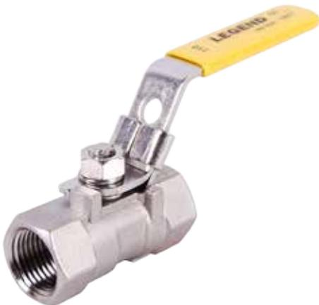
Compact, one-piece investment cast body design, 316 stainless steel body & end adaptor. Bottom-loaded blowout-proof stem, 316 stainless steel stem and ball. Equipped with a latch-lock handle (except 1/8" size), 304 stainless steel trim. Ideal for commercial or industrial applications where port size is not critical. Available in sizes & configurations: 1/8" - 2", FNPT x FNPT.
