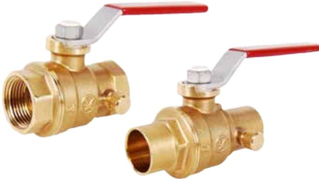
Maintenance-free, dual Viton® O-ring stem design, light weight and durable forged traditional brass body, blow-out proof stem, PTFE seats for improved wear. Ball with drain for maintenance or to prevent freeze. Dacromet® coated steel handle and nut for greater corrosion resistance. Available in sizes and configurations 1/2" - 1", FNPT x FNPT and 1/2" - 1", Sweat x Sweat.
