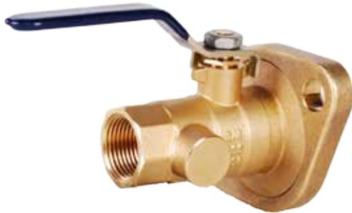
Traditional forged brass full port ball valve with flanged end for isolating circulator pumps. Standard flange connection rotates for positioning valve. Mounting holes are elongated to fit high velocity pumps. Configuration and Size: FNPT x Flange, Sweat x Flange, and 3/4", 1" and 1-1/4".
