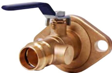
LegendPress™ press fitting end traditional forged brass full port ball valve with flanged end connection for isolating circulator pumps. Mounting holes are elongated to fit high velocity pumps. Standard flange connection rotates for positioning valve. Configuration and Size: Press Fitting x Flange, 3/4", 1" and 1-1/4".
