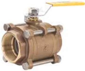
Large pattern three-piece cast bronze body and end adapters. Blow-out proof, forged brass stem. Chrome plated cast brass ball. PTFE seats (2), end adapter seals (2), stem seal, and stem packing. Packing nut is forged brass. Chrome plated steel handle with vinyl sleeve. AISI 304 stainless steel bolts, split washers and nuts (4 each).
