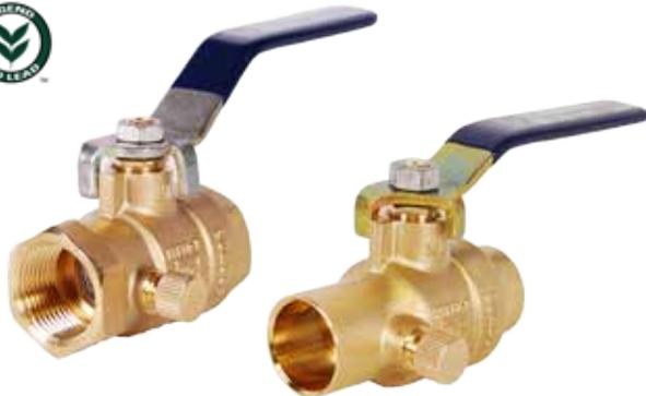
T/S-2102NL no lead brass full port ball valve with drain is ideal for maintenance and freeze protection. The EPDM O-ring and PTFE packing gland stem assures reliable and smoother operation requiring less torque. Constructed of no lead & DZR binary brass alloy. 1/2" - 1", FNPT x FNPT and 1/2" - 1", Sweat x Sweat.
