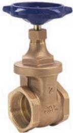
Cast bronze gate valve, screw over bonnet design, cast iron handle, full port, non-rising stem, integral seat and solid wedge.
