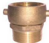
Forged brass, full-pattern body with double pin-lugs. Assorted sizes in Female NST thread pattern x Male NPT. Ball bearing swivel and includes washer.
