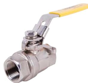
Full port ball valve; two-piece, 316 stainless steel investment casting; bottom-load blow-out proof stem; latch-lock handle; integral, tapped mounting pad for actuation or panel attachment.
