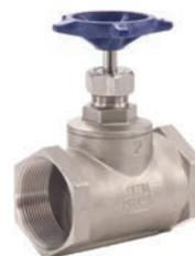
316 stainless steel, investment casting, rising stem, screw-in-bonnet, metal to metal seat and cast iron handle. Ideal for throttling.
