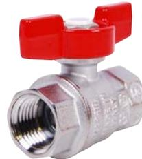
Maintenance free, dual Viton® O-ring stem design, lighter weight and durable forged body chrome plated, blow out proof stem, TFM-PTFE® seats for improved wear. Dacromet® coated steel handle and nut for greater corrosion resistance. Each valve is 100% factory pressure tested.
