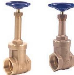
Rising stem, cast bronze, cast iron handle, full port, integral seat and solid wedge. T-416 is Class 150 and T-417 is Class 125.
