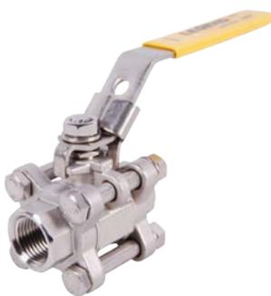
Full port ball valve; heavy-duty, three-piece 316 stainless steel investment casting; bottom-load blow-out proof stem; latch-lock handle; four 304 stainless steel nuts and bolts; body center lifts or swings out to permit servicing without end adapter removal.
