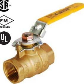
Full port ball valve with stainless steel ball and stem for greater strength, intended for frequent actuation. Includes latch lock steel handle and trim. Lockable in the full open and fully close positions.
