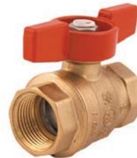
Maintenance free, dual Viton® O-ring stem design, lighter weight and durable forged body, blow out proof stem, TFM-PTFE® seats for improved wear. Each valve is 100% factory pressure tested.
