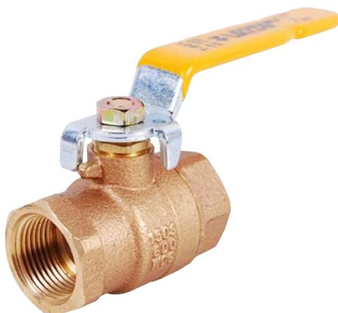
Large pattern, dezincification resistant, cast bronze body is ideal for underground water supply installations. Gland follower stem design with PTFE stem packing. Handle is chrome plated steel.
