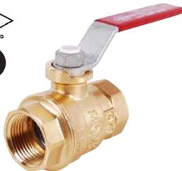
Maintenance free, dual Viton® O-ring stem design, lighter weight and durable forged body, blow out proof stem, TFM-PTFE® seats for improved wear. Dacromet® coated steel handle and nut for greater corrosion resistance. Each valve is 100% factory pressure tested.
