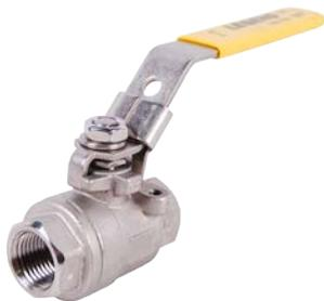
Large port ball valve; two-piece, 316 stainless steel investment casting; bottom-load blow-out proof stem; latch-lock handle; reinforced graphite impregnated seats; integral, tapped mounting pad for actuation or panel attachment.
