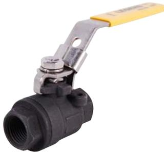
Two-piece, carbon steel investment casting; bottom-load blow-out proof stem; latch-lock handle; reinforced graphite impregnated seats; integral, tapped mounting pad for actuation or panel attachment.
