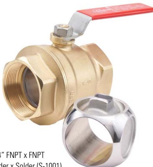
The cubic ball is designed to eliminate 90% of the surface area in contact with the seats to improve wear. This results in 20% reduction in torque and increases the life of the valve by 50%. Larger full body, six sided wrench flat, dual Viton® O-ring stem design, forged body, blow out proof stem, TFM-PTFE® seats for improved wear. Dacromet® coated steel handle and nut for greater corrosion resistance. Each valve is 100% factory pressure tested.
