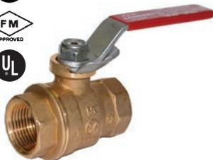
Maintenance free, dual Viton® O-ring stem design, lighter weight and durable forged body, blow out proof stem, TFM-PTFE® seats for improved wear. Dacromet® coated steel handle and nut; and lock shield. Lockable full open or full closed. Each valve is 100% factory pressure tested.
