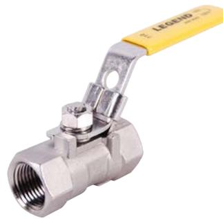
Reduced port ball valve; one-piece, 316 stainless steel investment casting; bottom-load blow-out proof stem; latch-lock handle; and ideal for commercial or industrial applications.
