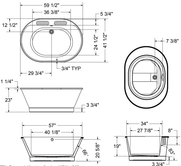
(:) Recommended faucet area 2 sections of 12" (L) x 4" (W). Depth recommended for straight pipes 8".
