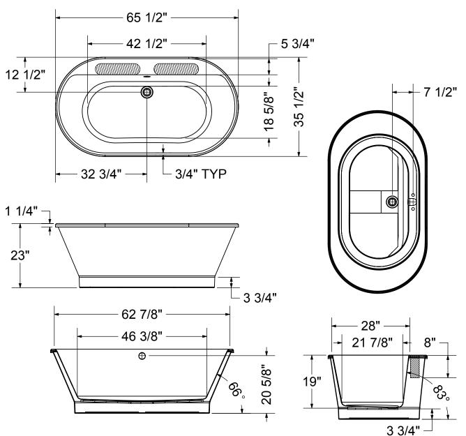
(:) :Recommended faucet area 2 sections of 16" (L) x 4" (W). Depth recommended for straight pipes 8".
