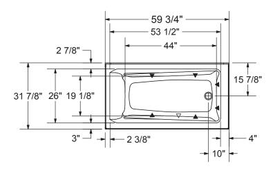
1" Single Integrated tiling flange (shown) 2" Double Integrated tiling flange (not shown) Drop-in model (Shown)
