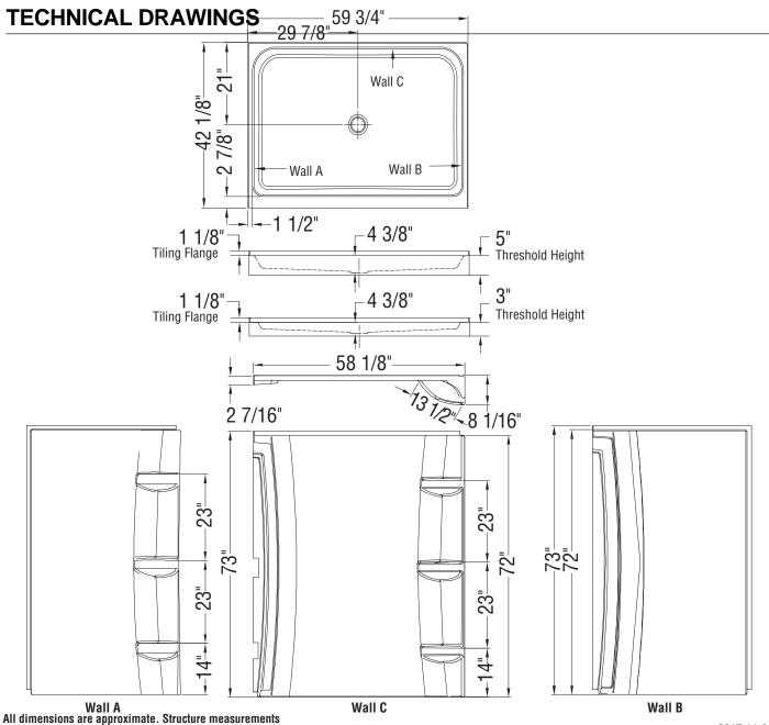
must be verified against the unit to ensure proper fit.
