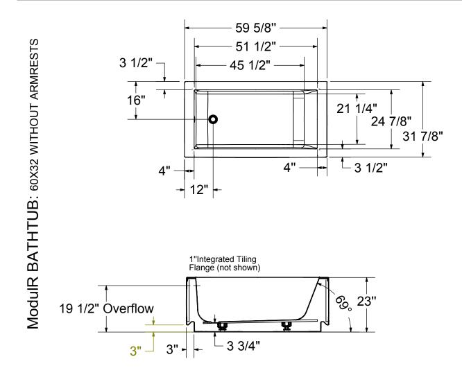
This technical drawing is universal for all ModulR bathtub configurations. (Left/Right Corner & Wall-mounted)
