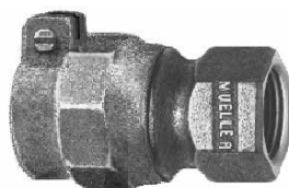
Straight coupling Mueller Pack Joint Connection for CTS O.D.* tubing x F.I.P. thread
