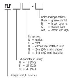
\* Lid insulation has an R-value of 10 per 2-inch (50-mm) increment Note: For fiberglass basin bottoms without holes, order FLF18 or FLF21
