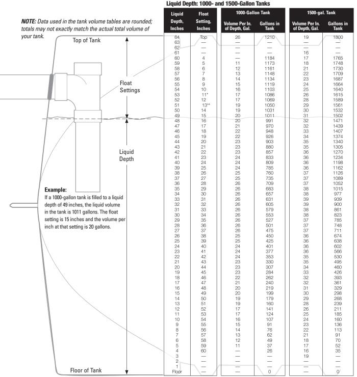
\* The invert of inlet is typically set 11 inches down from the top of the tank, or in accordance with prevailing state or local regulations. \*\* For gravity discharge applications, the invert of the outlet is typically located 13 inches down from the top of the tank.
