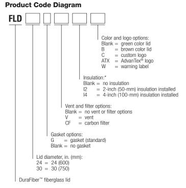
\* Insulation has an R-value of 10 per 2-inch (50-mm) increment.
