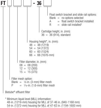
48-in. (1219-mm) housing for MLL of 37-46 in. (940-1168 mm) 54-in. (1372-mm) housing for MLL of 47-63 in. (1194-1600 mm) 60-in. (1524-mm) housing for MLL of 64-84 in. (1626-2134 mm) 66-in. (1676-mm) housing for MLL of 85-112 in. (2159-2845 mm)
