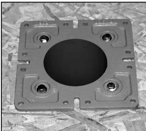
**PASCO's** NEW Quick Set Square Closet Flange will solve the problem of properly supporting a closet flange mounted in a square hole. Keep in mind that the pipe doesn't support the flange, the sub-floor does. Simply push the QUICK SET CLOSET FLANGE flush on the DWV pipe and alternately tighten the four stainless steel screws. Secure to subfloor with brass wood screws.
