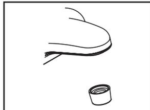
(4) Important: After installation is complete, remove aerator. Turn water supplies on and allow both hot and cold water to run at least one minute each. While water is running, check for leaks. Turn off water and replace aerator.
