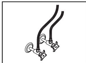
(3) Connect both hot (left) and cold (right) flex inlet lines to water supply valves. Note: Additional adapters or flex supply lines are required if outlet size of water supply valve is not 3/8" compression.
