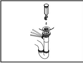
(6) Push pivot rod down, insert drain plug carefully. Test to ensure drain plug works properly.
