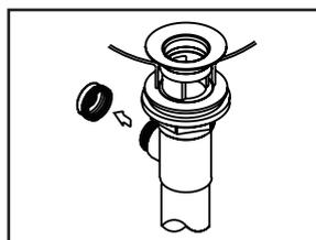
(5) Remove pivot rod nut from pop-up body, ensure the washers is in place, insert pivot rod, tighten pivot rod nut back to pop-up body.
