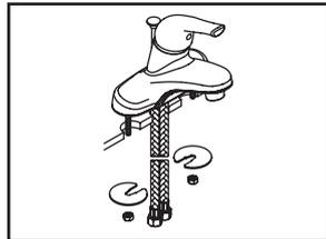
(2) Apply adequate plumbers putty along the boundary of base gasket. Thread mounting bolts to the bottom of faucet. Carefully lead both stainless steel flex inlet lines through center mounting holes, align faucet on the mounting surface. Slide mounting plate to the mounting bolts from underneath of the sink and thread mounting nut onto mounting bolts. Tighten mounting nut with help of basin wrench or adjustable wrench.
