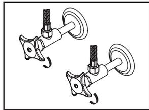
(1) Shut off water supplies. Remove old faucet. Clean mounting surface in preparation for new faucet.
