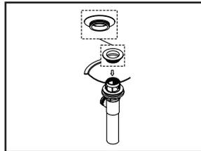
(2) Place a ring of putty on the bottom of flange.
