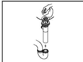
(4) Remove the excess putty. Connect the trap (check manufacturer's instructions for installation)
