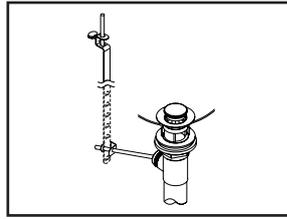
(7) Connect lift rod strap to pivot rod by using clip. Tighten the thumbscrew to connect lift rod strap to pop-up lift rod.
