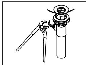
(3) Insert pop-up flange through drain hole and attach flange to body. Ensure the pop-up outlet faces towards the back of the sink. Tighten the locknut securely with a wrench. Do not overtighten.
