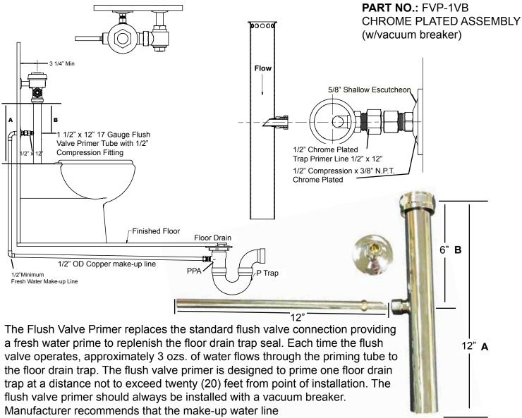
to the P-trap must have a continuous slope. (Consult Local Code Requirements).
