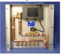
The Electronic Priming Assembly pictured is available in a single configuration but is capable of priming from twenty one to thirty separate floor drain traps from a single control unit. The manifold is available in either 1/2" or 5/8" compression, 1/2" PEX or PROPEX fittings. This model serves 21 to 30 drains.
