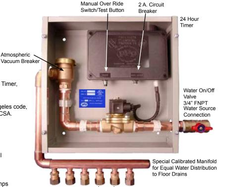
Tube Connection for Routing to Traps 1/2"/ 5/8" Compression
