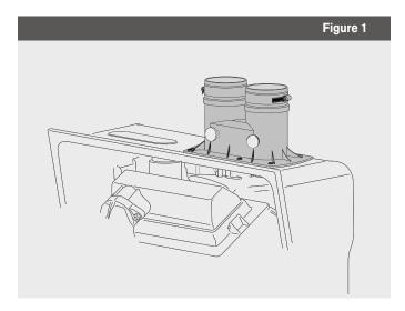
The polypropylene adaptor (p/n 8718600686) has an internal condensate drain which eliminates the need for an external condensate tee previously required with the aluminum vent adaptor.
