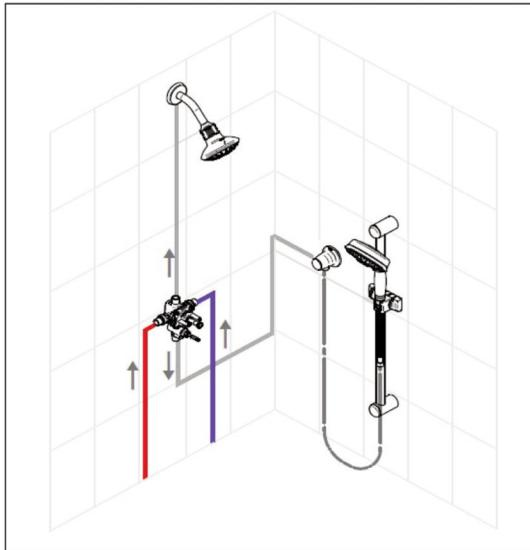
**ATTENTION:** Failure to use the outlet ports as indicated in either of these diagrams will void manufacturer's warranty
