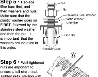
nuts are important to ensure a full-circle seal. Tighten nuts, starting with center bolts, alternating on either side of the sleeve. Gap between sleeve halves on either side should be the same when nuts are fully torqued.
