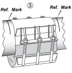
**Note:** If necessary because of flowing water, Steps 3 and 4 can be performed beside the pipe crack or hole. Slide the clamp over the break after the lifter bars have been snapped into place.
