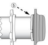
**Step 5** • Slide the GripRing up the pipe until its face is flush against the MJ gasket. For best results, orient the gap in the GripRing in the down position.
