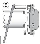
Equal distance must be maintained between the gland and the fitting throughout the installation, until the proper torque is achieved.
