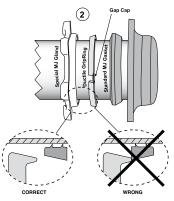
Note: Make sure that the tapered side of the GripRing faces the gland. This is very important, since the GripRing taper engages the taper in the gland. 10 & 12" GripRings have a Gap Cap. Do not remove Gap Cap.
