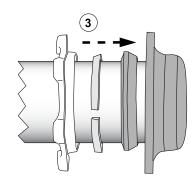
Step 4 • Slide the gasket into the MJ bell pocket as far as possible. The gland (and GripRing) may be used to tap the gasket into place if required. Be sure that the gasket is properly seated and fully pressed into the gasket recess.
