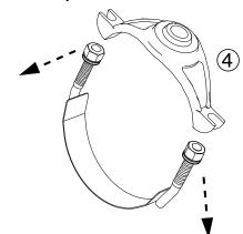
**Step 5** • Position the saddle body on the pipe such that the outlet is in the correct location.
