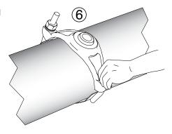
**Step 7** • Tighten all nuts evenly in 15-20 ft-lbs. increments. Use a wrench with at least a 12 inch handle.
