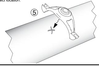
Step 6 • Install strap(s) on saddle body, and tighten finger tight. Make sure the gasket has seated itself flat onto the pipe face.
